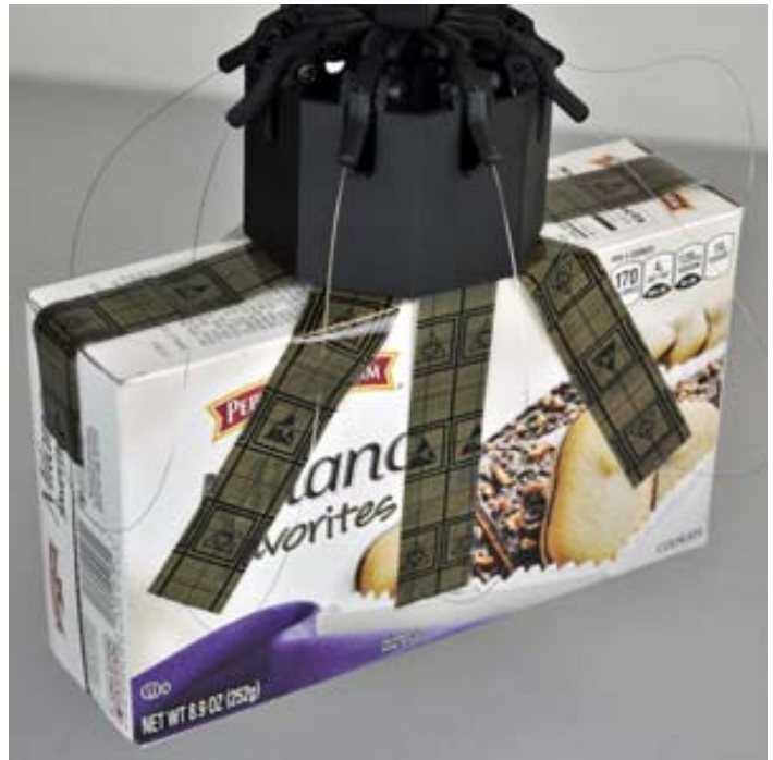
Grabit's gripper has flexible electrostatic appendages.
