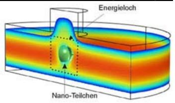
Cross-section through two chip-sized glass plates in which a nanoparticle is trapped in an energy hole (or "potential well" to use the scientific term). The colored fields show the different charges in the electrostatic field. The red zone signifies a very low charge, while the blue edges have a strong charge. vaccines and numerous pharmaceuticals. "The charge of the particles plays a major role in this," the Zurich-based scientist tells us.
