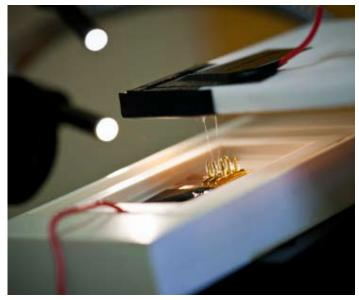
A tiny array of silicon tips sandwiched between electrodes spins out "nanofibers" of plastic that could be useful for a host of applications.
