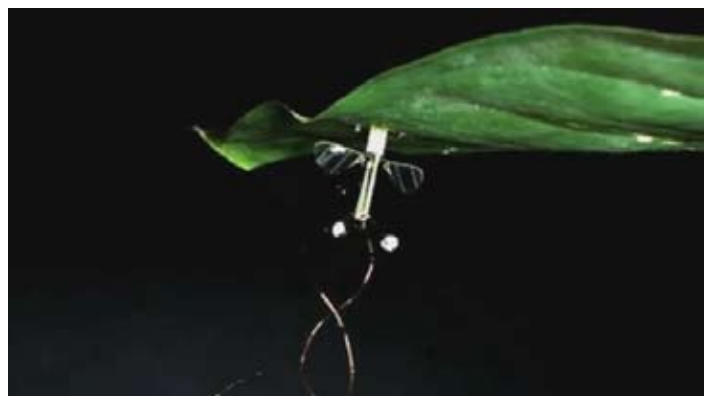
The RoboBee uses electrostatic attraction to stick itself under almost any surface, including wood, glass and even leaves. (Harvard University)
