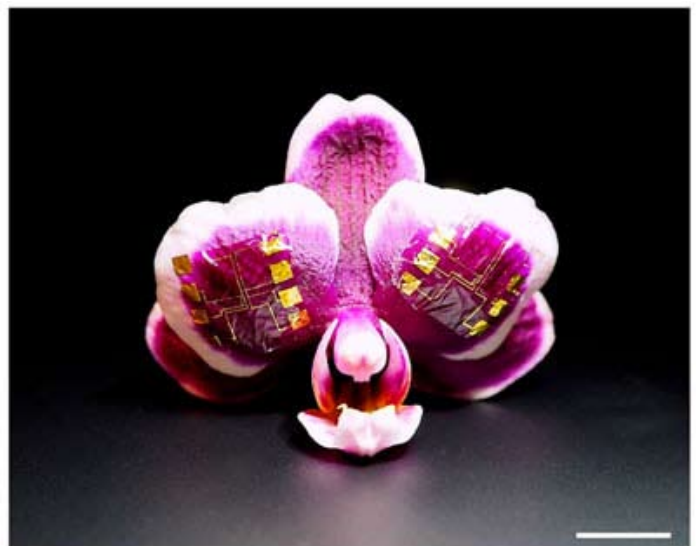
Figure: IGT-based NAND and NOR gates conform to the surface of orchid petals (left). Scale bar, 1cm. Optical micrographs of NOR (upper right) and NAND (lower right) logic gates. Input (I1, I2) and output (O) configuration is indicated. Scale bar, 100 \mu\text{m} .
