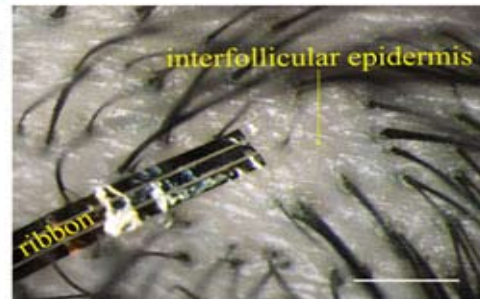
Figure 4: Optical micrograph of μ-EEG IGT conforming to human scalp; devices were designed to fit the interfollicular epidermis. Scale bar 2 mm.
