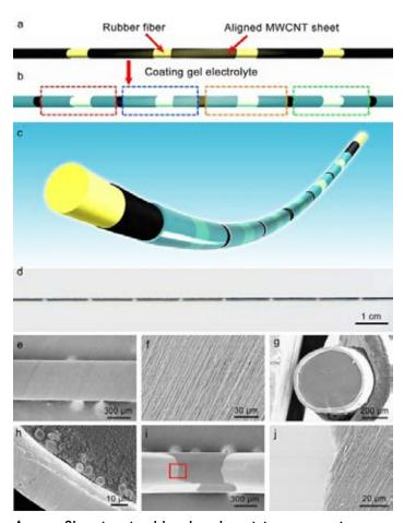
A new fiber inspired by the electricity-generating cells in electric eels could power wearable devices. The fibers (shown in the schematic above) combine conducting carbon nanotubes with insulating rubber wires and electrolyte gel to create tiny capacitors. The capacitors are placed in series to generate large voltage. At bottom, scanning electron micrograph images of the new fibers. Credit: H. Sun et al, Advanced Materials
