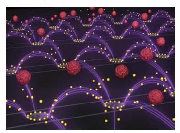
An artist's representation of the nanoparticle removal chip developed by researchers in Professor Michael Heller's lab at the UC San Diego Jacobs School of Engineering. An oscillating electric field (purple arcs) separates drug-delivery nanoparticles (yellow spheres) from blood (red spheres) and pulls them towards rings surrounding the chip's electrodes. The image is featured as the inside cover of the Oct. 14 issue of the journal Small. Image credit: Stuart Ibsen and Steven Ibsen.
