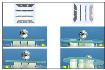
sheets in a plane, and once the sheets were aligned On a mechanical oscillator, a glass stage featuring a metal sphere on a tee was supported by three cylindrical pillars of magnetically structured hydrogel containing cofacially oriented TiNSs (0.8 wt%) in parallel (g) or orthogonal (h) direction to the cylinder cross-section.
