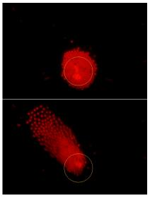
These images were taken from a video illustrating a new technique that uses a laser and holograms to precisely position clusters of numerous tiny particles within seconds, representing a potential new tool to analyze biological samples or create devices using "nanoassembly." The red dots are individual particles.
