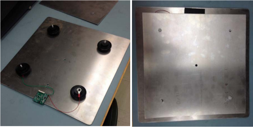
Fig. 2. ARL custom printed circuit board connected to the 0.010-m 2 top and 0.134-m 2 bottom aluminum plates, held securely by plastic screws and 3D-printed spacers (left). The completed Smart D-dot sensor with custom enclosure ensures the circuit does not contact either plate (right).
