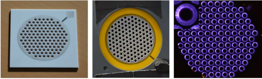
Fig. 18. Photographs of the plasma discharge array prototype (left), mounted at the jet exhaust (center) and powered by an AC voltage with peak amplitude of 7 \text{ kV}_p at 2000 Hz.
