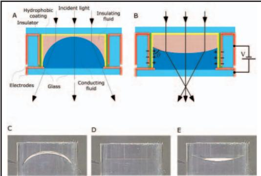
(A) Schematic cross section of the FluidFocus lens principle. (B) When a voltage is applied, charges accumulate in the glass wall electrode and opposite charges collect near the solid/liquid interface in the conducting liquid. The resulting electrostatic force lowers the solid/liquid interfacial tension and with that the contact angle? and hence the focal distance of the lens. (C) to (E) Shapes of a 6-mm diameter lens taken at different applied voltages.
