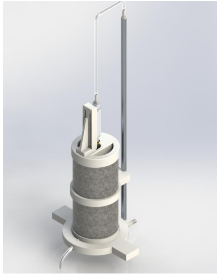
Figure 5. Solidworks rendering of the test chamber.
