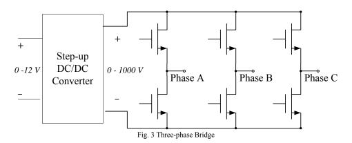
The digital signal controller controls which transistors are on, creating three square waveforms, each shifted  $120^{\circ}$  of another. The three square waveforms are illustrated in *Fig. 4*.
