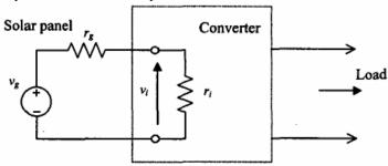
Fig. 6 Solar Panel with DC-DC Converter
