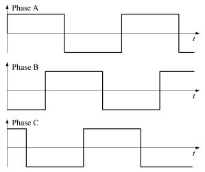
Fig. 4 Three-phase Square Waveforms
