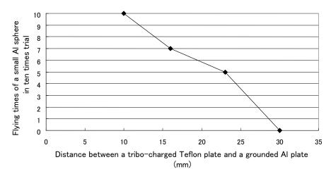
Fig. 9. Flying times of a small Al sphere in ten times trial vs. distance between a tribo-charged Teflon plate and a grounded Al plate.
