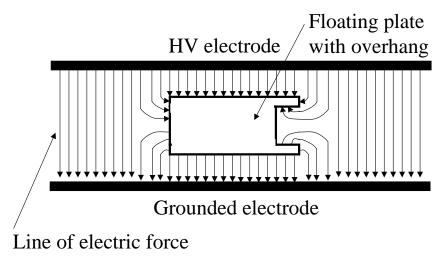
Fig. 4. Lines of electric force around the floating plate with overhangs which is placed center between the high voltage applied upper electrode and the grounded lower electrodes.
