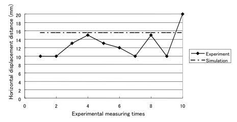
Fig. 12. Horizontal displacement distance of the right open Al cubic box vs. experimental measuring times.
