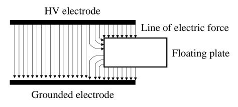
Fig. 2. Lines of electric force around the floating plate which is inserted by half between the high voltages applied upper electrode and the grounded lower electrodes.
