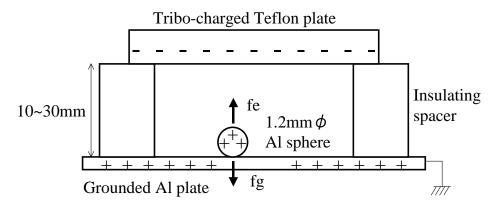
Fig. 8. Schematic diagram of the surface charge density measuring instrument of the tribo-charged Teflon plate
