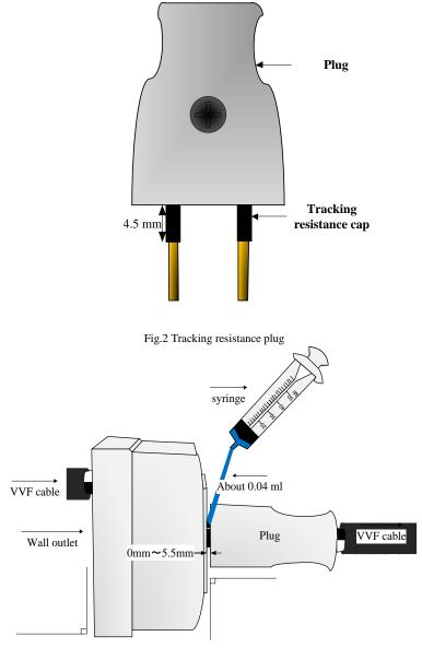
Fig.3 The representation of the experiment setup
