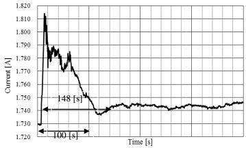
Fig.5 The effective value of the current in the gap length of 4.50 mm
