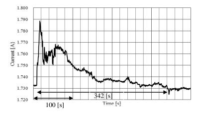
Fig.6 The effective value of the current in the gap length of 5.50 mm
