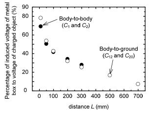
Fig. 8. Percentage of the induced voltage of an ungrounded metal box to the voltage of charged body at the distance L.
