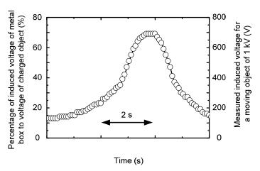
Fig. 5. Measured induced voltage when a charged body of 1 kV moves at the distance L of 10 mm.
