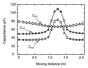
Fig. 3. Measured capacitances of  $C_{\rm m1}$ ,  $C_{\rm m2}$ , and  $C_{\rm m3}$  for body-to-ground at the distance L of 10 mm.
