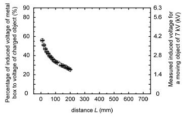
Fig. 6. Percentage of the induced voltage of an ungrounded metal box to the voltage of charged body and measured induced voltage when a charged body of 7 kV moves at the distance *L*.
