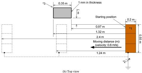
Fig. 1. Arrangement of experimental setup. The distance *L* denotes the distance between the charged body (object) and the front of metal box.\*1: charged body, \*2: DC high voltage power supply (0-50 kV), \*3: metal box, \*4: acrylic table (PMMA), \*5: automatically transporting stage, \*6: grounded copper plane, \*7: electrostatic measuring device (711, 3M Co.), \*8: oscilloscope (U1604A, Agilent Co.).
