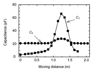
Fig. 2. Measured capacitances of  $C_1$  and  $C_2$  for body-to-body at the distance L of 10 mm
