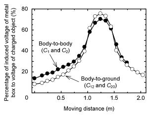
Fig. 7. Percentage of the induced voltage of an ungrounded metal box to the voltage of charged body at the distance L of 10 mm.
