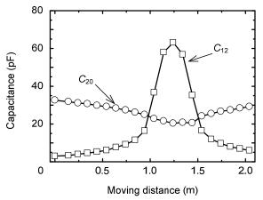
Fig. 4. Calculated capacitances of  $C_{12}$  and  $C_{20}$  for body-to-ground at the distance L of 10 mm.
