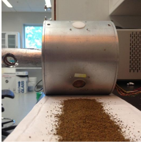
Fig. 1. - WES prototype prepared to roll on Martian regolith simulant. The circular insulators are shown protruding from the surface of the wheel.
