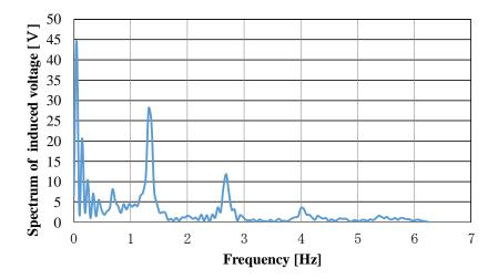
Fig.3. Frequency spectrum of walking motion
