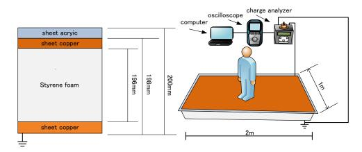
Fig.1. Experiment layout drawing
