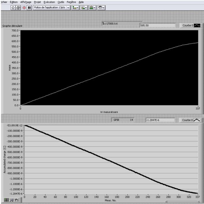
Fig. 3. Charge (a) and mass (b) evolution, recorded by the virtual instrument developed in LabView
