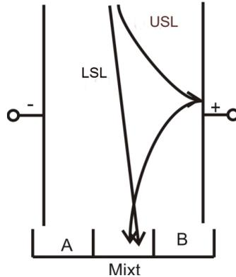
Fig. 1. Trajectories of granules charged beyond the upper specification limit (USL) and or below the lower specification limit (LSL), in a free-fall tribocharging separator.
