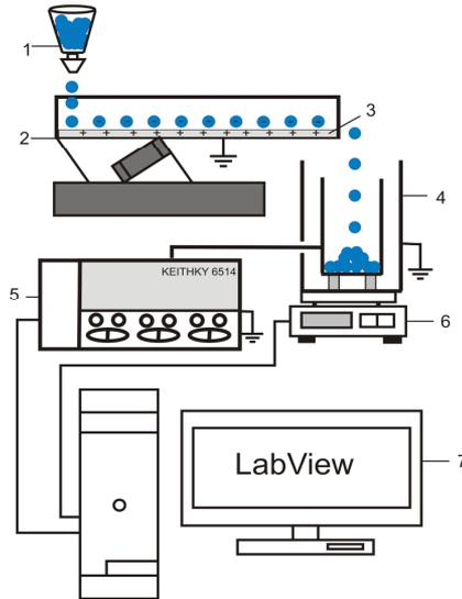
Fig. 2. Schematic representation of the experimental set-up for the study of tribocharging process of granular materials: 1 – vibratory device for feed rate control, 2- vibratory feeder tribocharging device, 3 – PET sheet on the vibratory feeder tray, 4 – Faraday pail, 5 – Keithley electrometer, 6 – electronic scale, 7 – computer.
