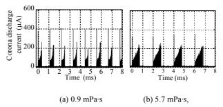
Fig. 2. Time variation of pulse groups in corona discharge occurring from the tip of a water droplet with various viscosity
