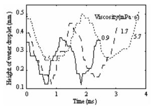
Fig. 8. Time variation of the height of a viscous water droplet during resonant vibration.
