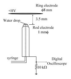
Fig. 1. Arrangement of a ring to capillary electrode system to occur corona discharge from at the tip of water drop.
