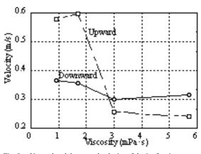
Fig. 9. Upward and downward velocity of thetipof a viscous water droplet during resonant vibration.
