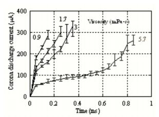
Fig. 5. Time variation of mean peak value of corona pulse group in a single deformation
