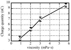
Fig. 6. Relation between viscosity of water and charge quantity of corona pulse train
