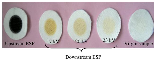
Fig. 9. Photographs of the filter samples
