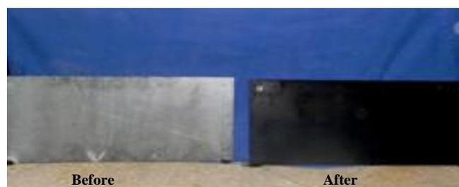
Fig. 10. Photographs of the collecting electrodes before and after gas treatment
