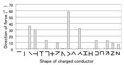
Fig. 11. Simulated direction of the force that acts on 19 different shape charged conductors
