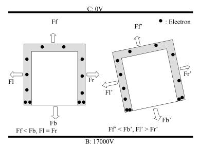
Fig. 19. Charge distribution and electrostatic forces of the charge carrier in normal and declined conditions
