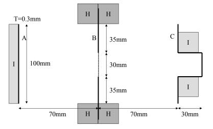
Fig. 17. Plane view of the experiment instrument of the new electrostatic generator
