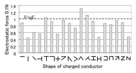
Fig. 9. Simulated magnitude of the force that acts on 19 different shape charged conductors
