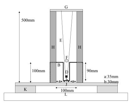
Fig. 16. Side view of the center of the experiment instrument of the new electrostatic generator
