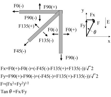
Fig. 8. Calculation procedure of magnitude and direction of the electrostatic force that acts on No.17 charged conductor
