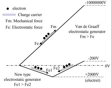
Fig. 14. Schematic explanation of principle of two electrostatic generators
