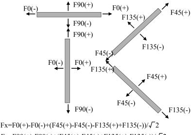
$$Fy=F90(+)-F90(-)+(F45(+)-F45(-)+F135(+)-F135(-))/\sqrt{Fig. 7 Eight directions of the forces that act on the 19 charged conductors$$
