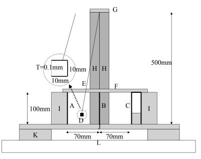
Fig. 15. Front view of the experiment instrument of the new electrostatic generator
