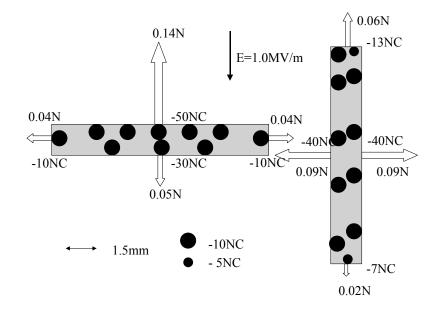
Fig. 10. Charge distribution and electrostatic forces on surfaces of a solo horizontal plate and a solo vertical plate.
