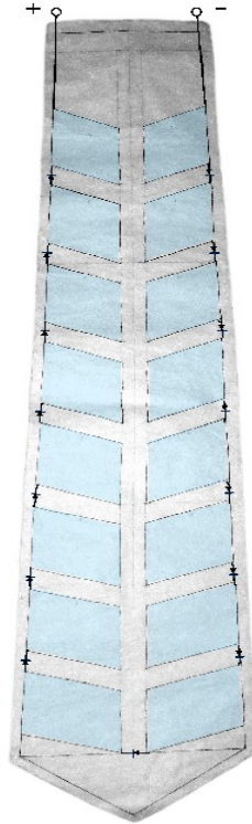
Fig. 7: Sp4rk13 skirt panel pattern. Panels were fabricated using similar materials and techniques as in the prototype panel but on a larger scale (16 electrodes with a total area of about 156 \text{ in}^2 (\approx 0.1 \text{ m}^2) ). Terminal electrodes (+ and -) were fabricated of folded conductive organza to make robust sewable attachments.
