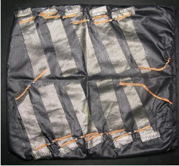
Fig. 3: Inside view of prototype skirt panel. 10 electrodes (each approximately 2.5\text{ cm} \times 10\text{ cm} ) were cut out of conductive organza and affixed to the nylon substrate using spray fabric adhesive. Diodes were soldered to sections of copper braid and sewn across the organza strips. Two additional sections of copper braid were sewn to the terminal electrodes to allow connection to external circuitry.
