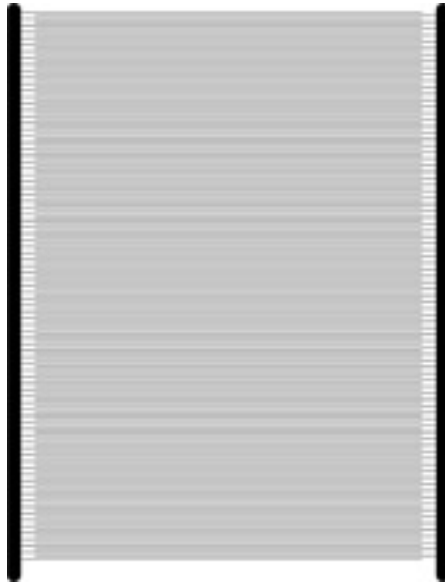
Fig. 4. EDS installed on the PEM door. Two sets of parallel copper electrodes in an interlaced comb configuration are embedded between two sheets of Kapton™ film.
