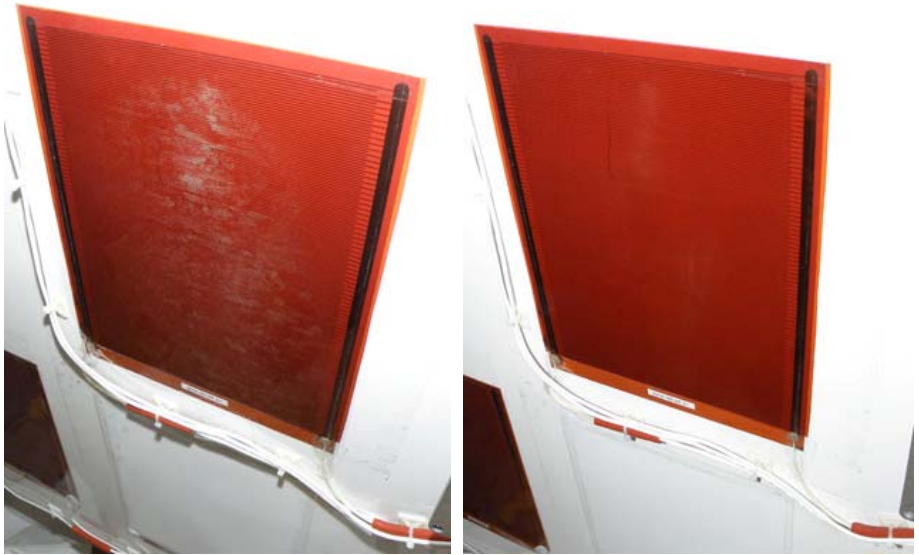
Fig. 7. Post installation tests of the 20 cm \times 25 cm EDS. JSC-1A simulant dust was thrown at
