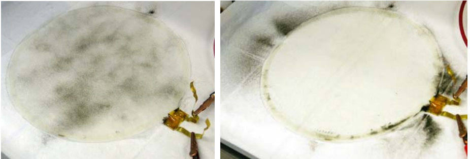
Fig. 6. Photographs of the 20-cm diameter transparent EDS for the PEM viewport during laboratory tests. JSC-1A simulant dust was deposited in a relatively uniform fashion, as shown on the left. The photograph on the right shows the EDS after activation. Dust has been removed to the region outside the electrode grid. These tests were performed with the EDS sitting horizontally in a glove box.
