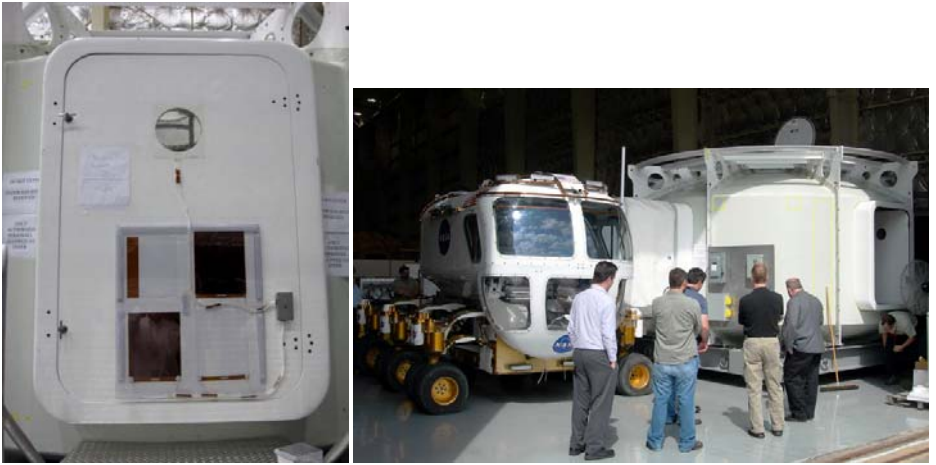
Fig. 3 (a). One of the PEM doors with the EDS systems installed. (b) The Lunar Electric Rover mated to the PEM.
