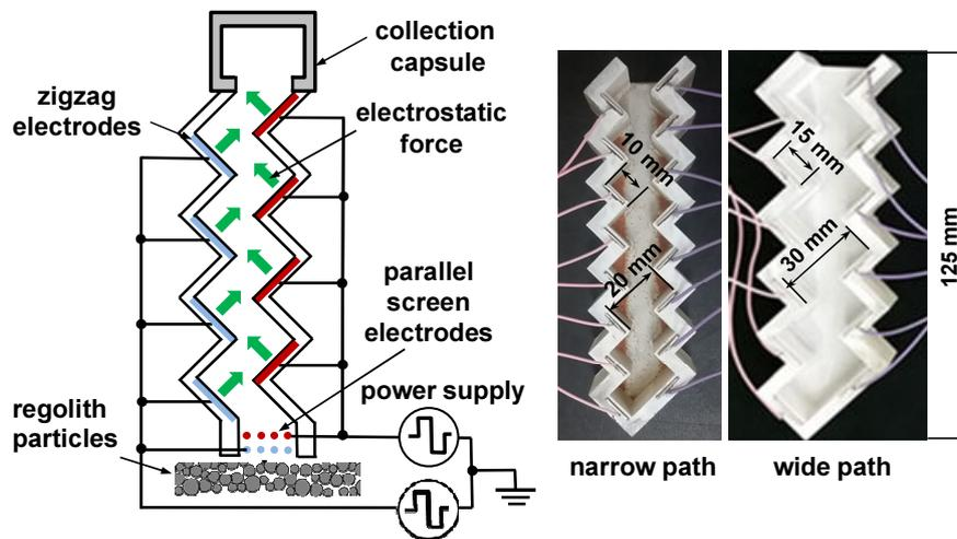
Fig. 1. Schematic illustration of the sampling system (left) and photographs of the zigzag path for transporting regolith particles (right).
