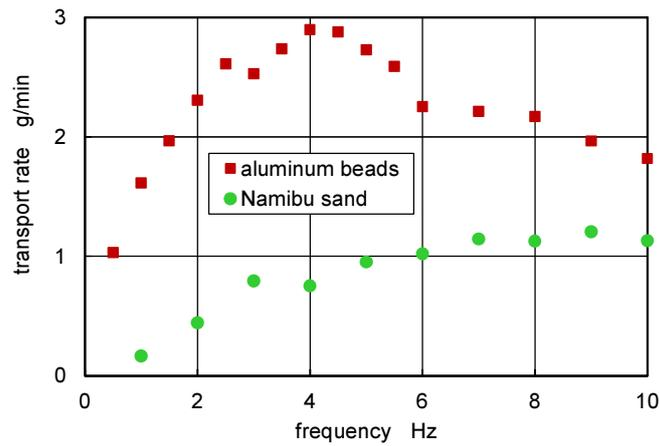
Fig. 5. Transport rate of particles with respect to the frequency of applied voltage (narrow path, 8 kV<sub>p-p</sub>).
