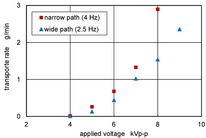
Fig.3. Transport rate of particles with respect to the applied voltage (aluminum beads, 8 kV<sub>p-p</sub>).
