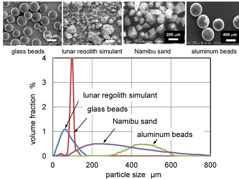
Fig. 2. SEM images of particles used for experiment and their particle size distributions.
