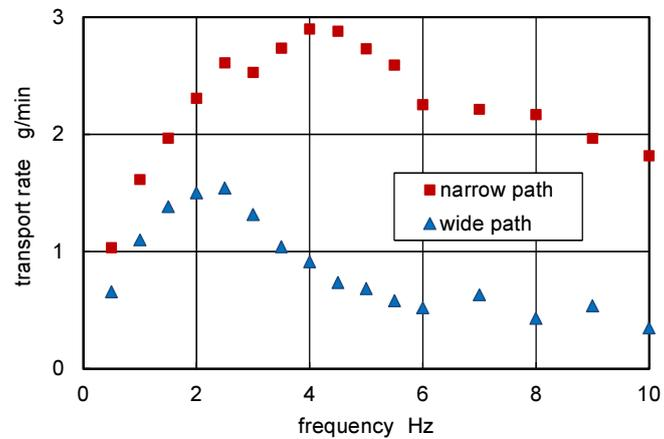
Fig. 4. Transport rate of particles with respect to the frequency of applied voltage (aluminum beads, 8 kV<sub>p-p</sub>).
