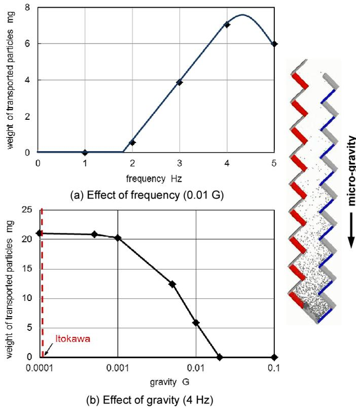
Fig. 6. Calculated performance in space (narrow path, 8 kV<sub>p-p</sub>). The figure on the right shows a calculated snapshot of particle transport in micro-gravity and vacuum environment.
