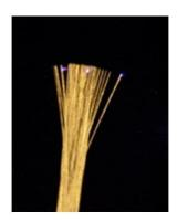
Figure 1 Bundle of fine metal fibers (100 fibers of 12 µm diameter made of stainless steel)
