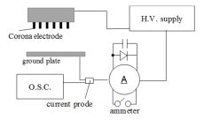
Figure 2 Measuring circuit
