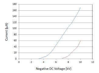
Figure 3 Voltage-current characteristics of the bundle and the needle electrode
