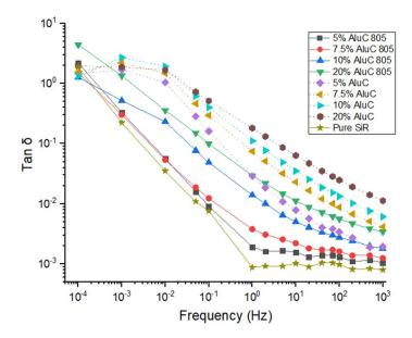
Fig. 2. Tan  $\delta$  for treated and untreated nano-alumina filled SiR at different weight percentages and pure SiR as a function of frequency.
