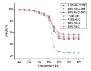
Fig. 3. TGA result of treated and untreated nano-alumina.
