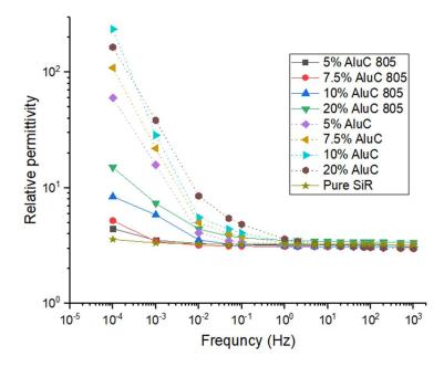
Fig. 1. Relative permittivity for treated and untreated nano-alumina filled SiR at different weight percentages and pure SiR as a function of frequency.
