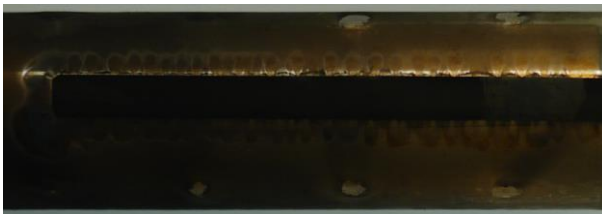
Fig. 5. Photo of the glass tube surface taken after 160 min of operation shown in Fig. 5 (the center horizontal strip seen is one of the surface discharge electrodes)
