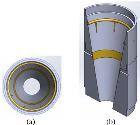
Fig. 2 An EHD gas pump with a diameter ratio of 1/3, (a) top view, (b) cross-sectional view.
