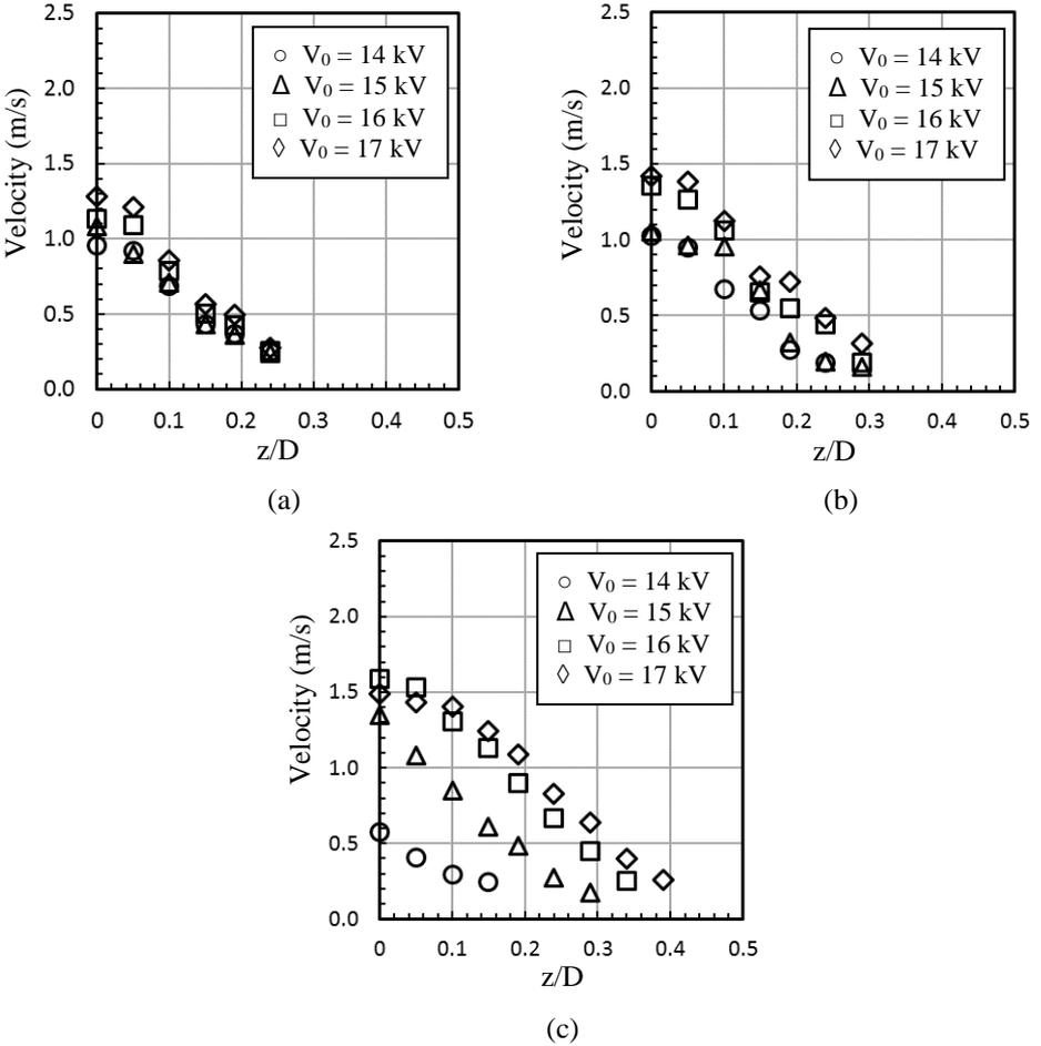
Fig. 6 Velocity profiles of the corona jet produced by nozzles with various diameter ratios (at  $z/D = 2$  from the nozzle exit), (a) DR = 1/4, (b) DR = 1/3, and (c) DR = 1/2.
