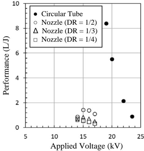
Fig. 8 Performance of the three EHD gas pumps examined.
