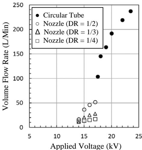
Fig. 7 Volume flow rate produced by the three EHD gas pumps examined.
