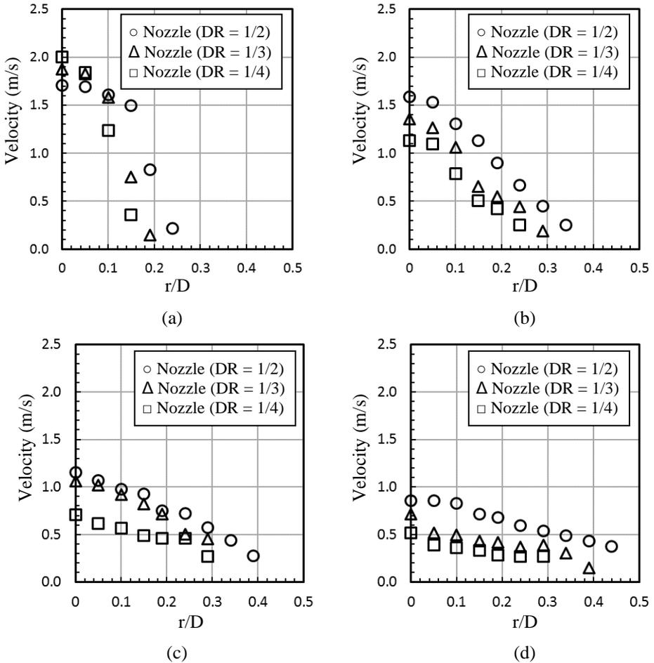
Fig. 5 Velocity profiles of the corona jet at various downstream distances from the nozzle exit ( $V_0 = 16$  kV), (a)  $z/D = 0$ , (b)  $z/D = 1$ , (c)  $z/D = 2$ , and (d)  $z/D = 3$ .
