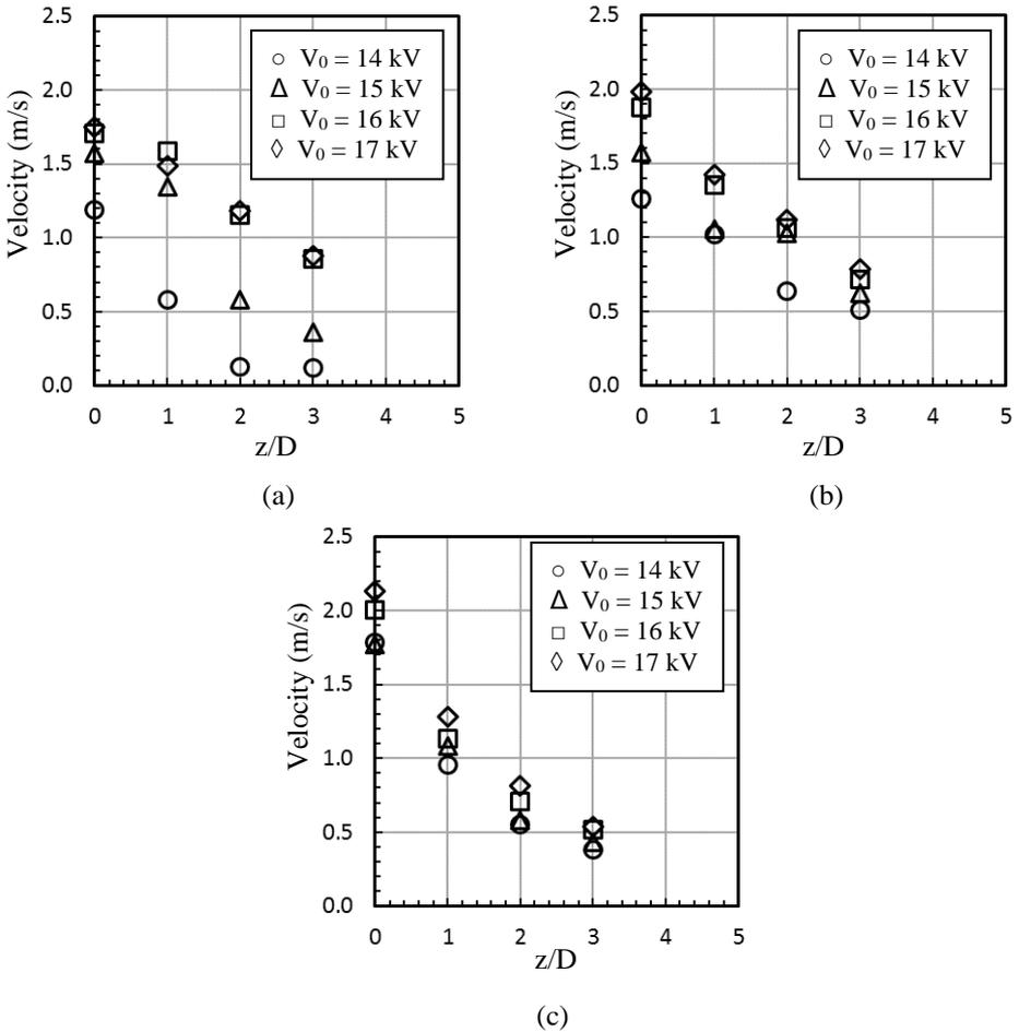
Fig. 4 Variation of the centerline velocity at various downstream distances from the nozzle exit, (a) DR = 1/2, (b) DR = 1/3, and (c) DR = 1/4.
