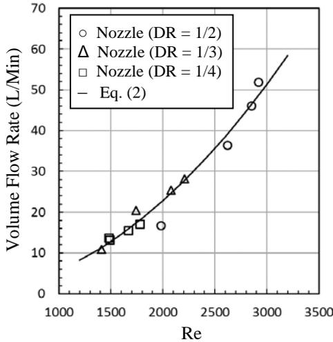
Fig. 9 Volume flow rate as a function of Reynolds number.
