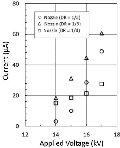
Fig. 3 Voltage-current characteristic curves of the EHD gas pumps.
