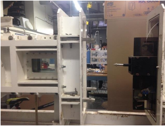
Fig. 3. Wind tunnel showing the test section (clear window on the left) and the internal sting on the right (with a standard aerodynamic cone attached) to which the electrode was mounted in this disassembled view.
