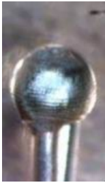
Fig. 2: Photo of a Thermocouple Weld. Picture shows the two thermocouple wires and the spherical bead.
