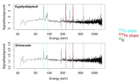
Fig 3. Gamma ray spectra, normalized against background and for mass, of ash samples from the two volcanic eruptions. Gamma peaks associated with particular natural decay chains are indicated in colour (cyan for  $^{238}$ U, red for  $^{232}$ Th and green for  $^{40}$ K)
