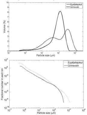
Fig 2. Size distributions of the ash samples used. (top) Volumetric size distribution, measured with a Malvern Mastersizer 2000. (bottom) Estimated number size distribution, calculated from the volumetric size distribution. Although spherical particles were assumed for simplicity, different packing fractions (0.5 for Eyjafjallajökull and 0.2 for Grímsvötn) were chosen to best represent the ash samples used.
