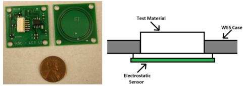
Fig. 5. Electrostatic sensor second generation prototype
