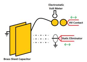
Fig. 11. Static eliminator test configuration
