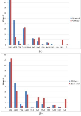
Fig. 2. Comparison of regolith simulants [11]
