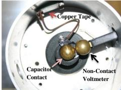
Fig. 13. Experimental setup for testing for the WES sensor geometry
