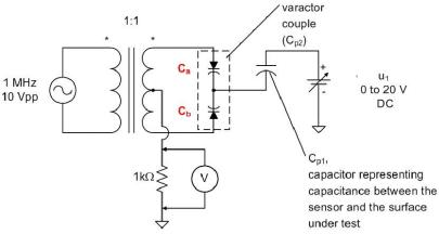
Figure 2. Varactor-based variable capacitance [12]
