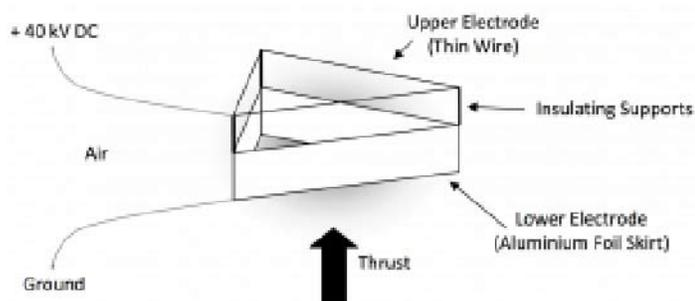
ed to the collector. As this cloud of ions moves toward the collector, it collides with surrounding neutral air molecules, pushing them along and creating a wind, or thrust.
