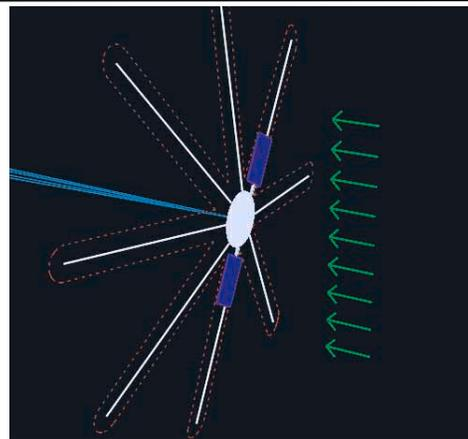
In this phase the wires have been deployed and the electron gun has been started. The blue lines symbolize the electron beam of the gun. The spinup propulsion arms and associated fuel tank have been jettisoned to save mass. The solar wind acts on the wires, bending them slightly. The electric field around the wires is depicted by dashed red line.
