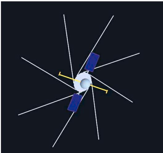
A schematic view of the deployment phase of a spinning electric sail. Only eight wires have been drawn for simplicity. The violet-blue surfaces are solar panels and the yellow lines are propulsive arms (with small rockets attached to the tips) which create the initial spacecraft spin.
