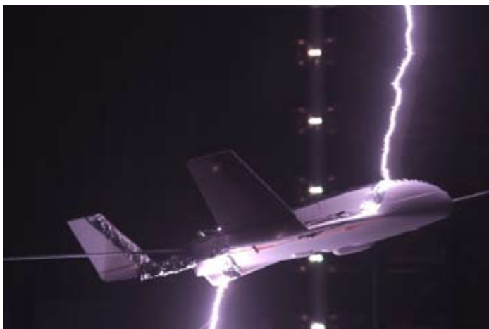
Lightning laboratory test on model aircraft. Image: Joan Montanya/Polytechnic University of Catalonia
