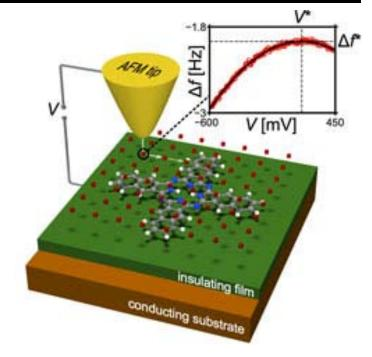
Schematic of the measurement principle. At each tip position, the frequency shift is recorded as a function of the sample bias voltage (inset, red circles). The maximum of the fitted parabola (inset, solid black line) yields the KPFM signal V\* for that position. Image courtesy of IBM Research - Zurich
