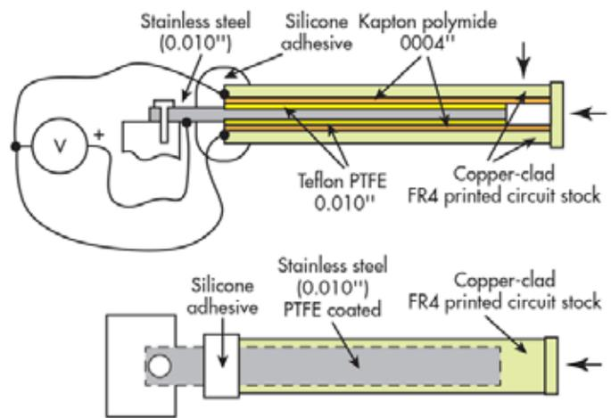
1. Construction of the triboelectric switch shows the layered implementation, which allows for rubbing and thus generation of high voltages.
