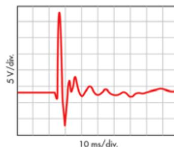
2. The peak voltage of the pulse obtained by tapping the switch depends on the force and speed of the finger tap, and the loading resistance (the probe impedance was  $10\text{ M}\Omega$ ).
