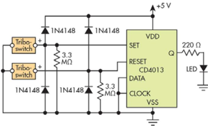
3. The demonstration circuit uses the switch to activate a simple LED; standard 1N4148 diodes are used as clamps to prevent high-voltage spikes from damaging the flip-flop IC.
