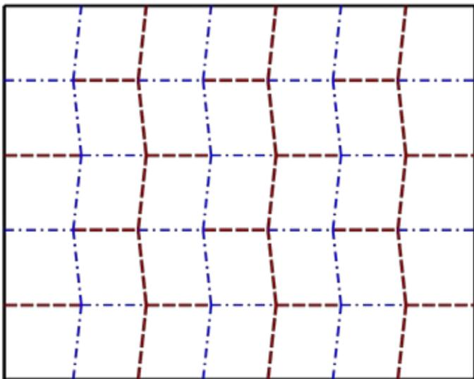
Crease pattern for a Miura fold. The parallelograms of this example have  $84^\circ$  and  $96^\circ$  angles. By Dmcq - Own work, CC BY-SA 3.0, <https://commons.wikimedia.org/w/index.php?curid=17473684>
