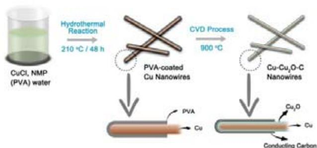
The three-layer coaxial nanocable contains a solid copper wire surrounded by a layer of copper oxide that is encased a layer of carbon just a few atoms thick.
