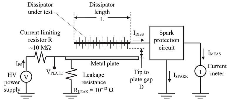
Fig. 3: The electrified metal plate simulates a charged target. The current from the dissipator is measured by the current meter that is protected by the spark protection circuit.
