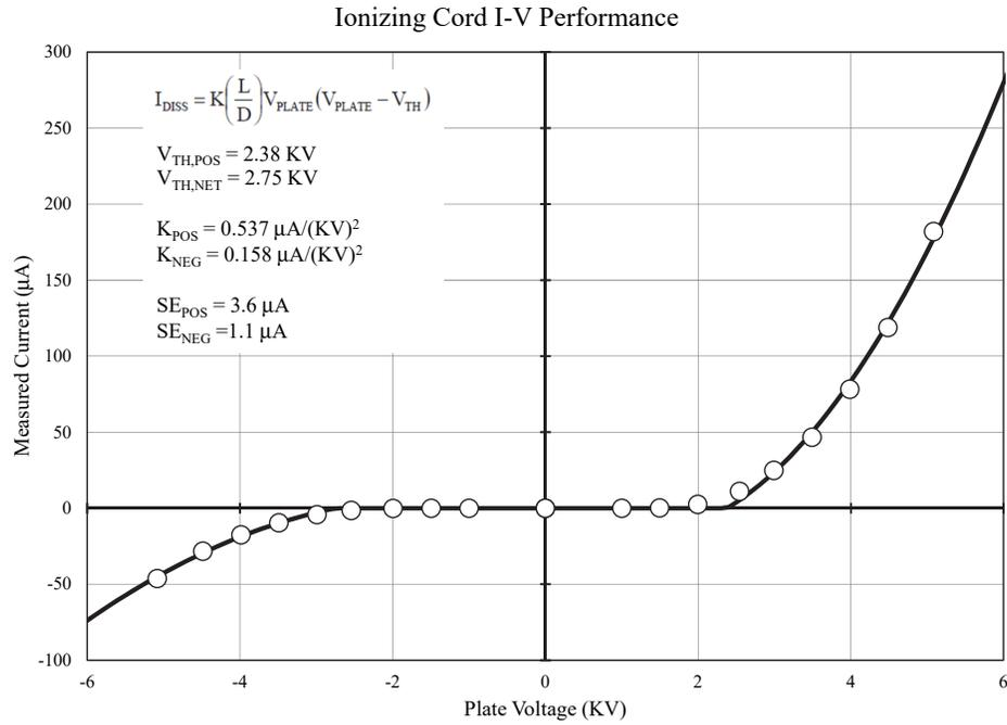
Fig. 5: The measured I-V data in Table 1 is fit with the empirical model in a least squares sense by adjusting the threshold voltage  $V_{\text{TH}}$  and constant  $K$ .
