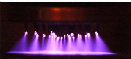
Fig. 2. (a) Corona image at 12 kV with reference line, (b) Intensity profile along the reference line
