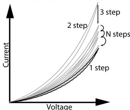
Fig. 2. Graphic illustration of the injection function estimation method by DCVC.
