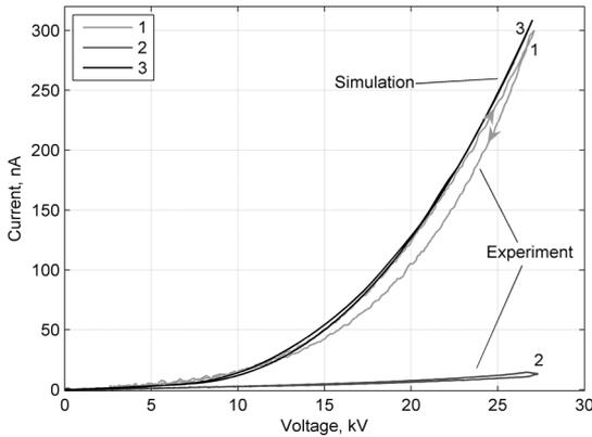
Fig. 3. Experimental DCVC for positive (curve 1) and negative (curve 2) polarity as well as DCVC obtained from the simulation (curve 3).
