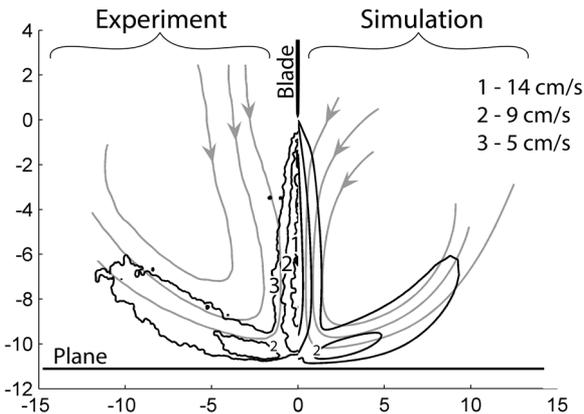
Fig. 4. Velocity field distribution in blade-plane electrode system in the case of experiment (left-hand side) and simulation (right-hand side).
