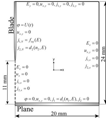
Fig. 1. Geometry of the computer model and boundary conditions.
