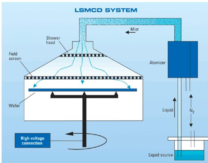
Schematic Diagram of Mist Deposition Apparatus
