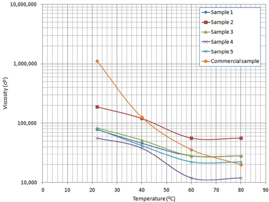
Fig. 1: Variation of viscosity of different formulations with increasing temperature.
