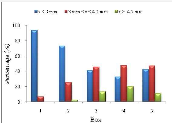
Fig. 11: Distribution of particle size in each collecting box for a 50% PVC / 50% HIPS sample.
