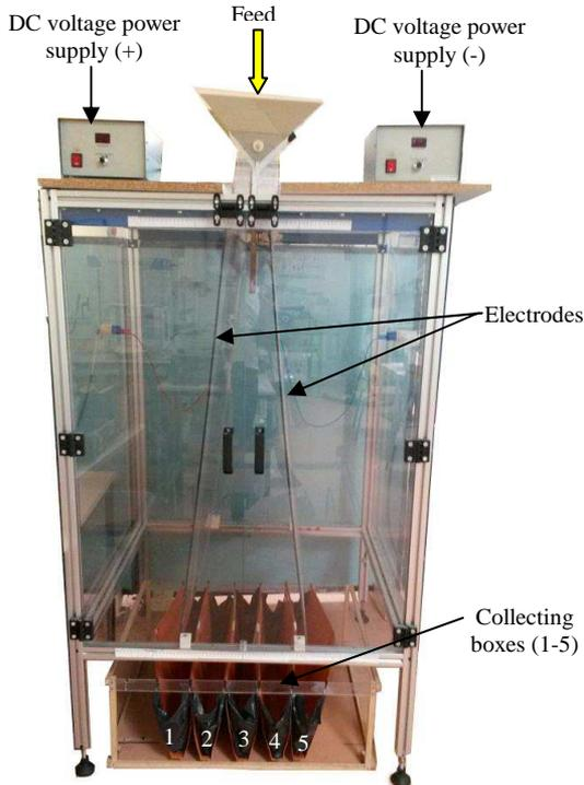
Fig. 2. The free fall electrostatic separator.
