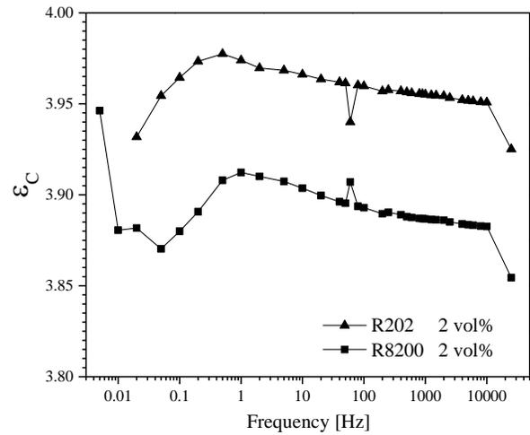
**Figure 5b.** Increments in relative permittivity of composites elaborated with R202 and R8200 nanosilica were observed for 2 vol% concentration.
