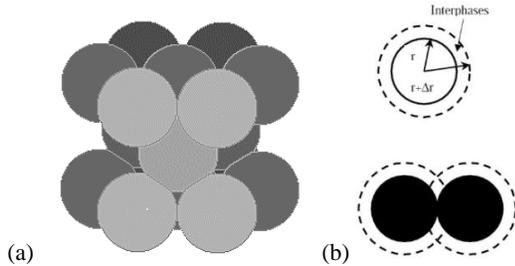
**Figure 3.** (a) The ABAB structure given the maximum filler volume fraction in a composite. (b) The interphase shell thickness  $\Delta r$  around the filler of radius  $r$  [10].
