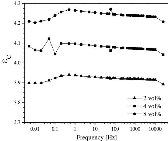
**Figure 5a.** Relative permittivity of the composites elaborated with R812 nanosilica at 2 vol%, 4 vol% and 8 vol%.
