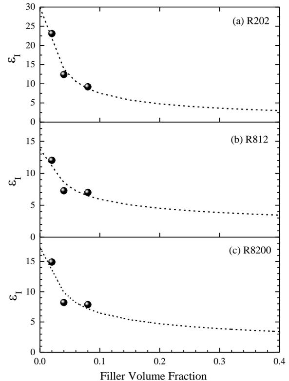
**Figure 8.** Predicted curves at 10 kHz for the relative permittivity of the interphase of silicone rubber composites made with (a) R202, (b) R812 and (c) R8200 nano silica. Circular dots represent the values obtained through experimental measurements and the dotted lines represent the theoretical  $\epsilon_I$  trend for the relative permittivity of the interphase in these systems.
