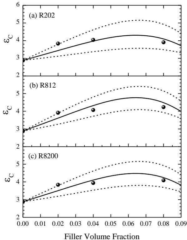
**Figure 7.** Predicted curves at 10 kHz for the relative permittivity of silicone rubber composites made with (a) R202, (b) R812 and (c) R8200 nano silica. Circular dots are the experimental values. The solid line represents the theoretical  $\epsilon_C$  and the dotted lines represent the upper and lower Wiener bounds.
