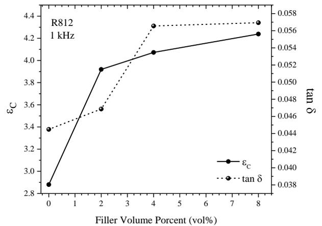
**Figure 6.** Variation of relative permittivity and dissipation factor of R812/silicone rubber nanocomposites at 1kHz.
