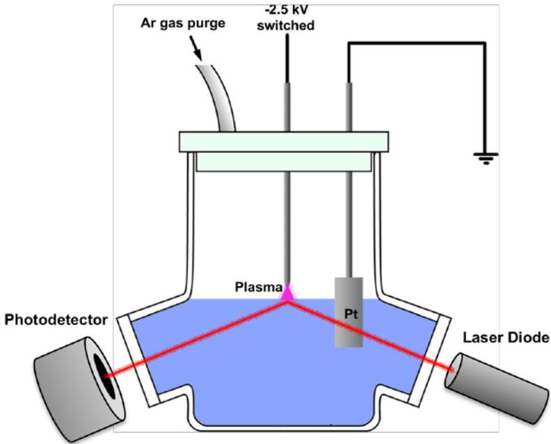
Fig. 1 Shown above is a schematic of the experimental setup for optically measuring solvated electrons. A laser diode is focused onto the plasma-liquid interface. The angle of incidence is greater than the critical angle for total internal reflection, so the beam is entirely reflected into the detector sans the small amount absorbed by solvated electrons.
