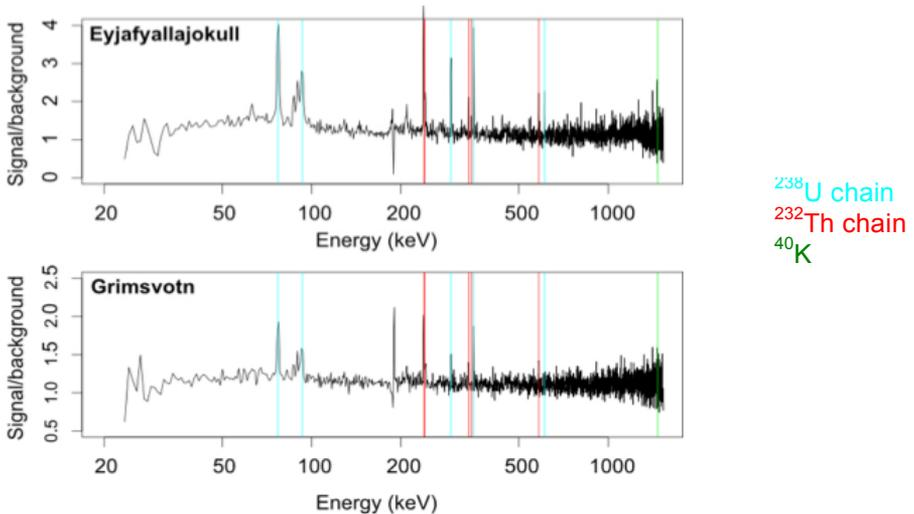
Fig 3. Gamma ray spectra, normalized against background and for mass, of ash samples from the two volcanic eruptions. Gamma peaks associated with particular natural decay chains are indicated in colour (cyan for  $^{238}\text{U}$ , red for  $^{232}\text{Th}$  and green for  $^{40}\text{K}$ )
