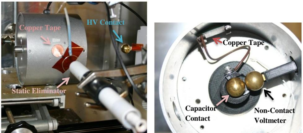
Fig. 13. Experimental setup for testing for the WES sensor geometry
