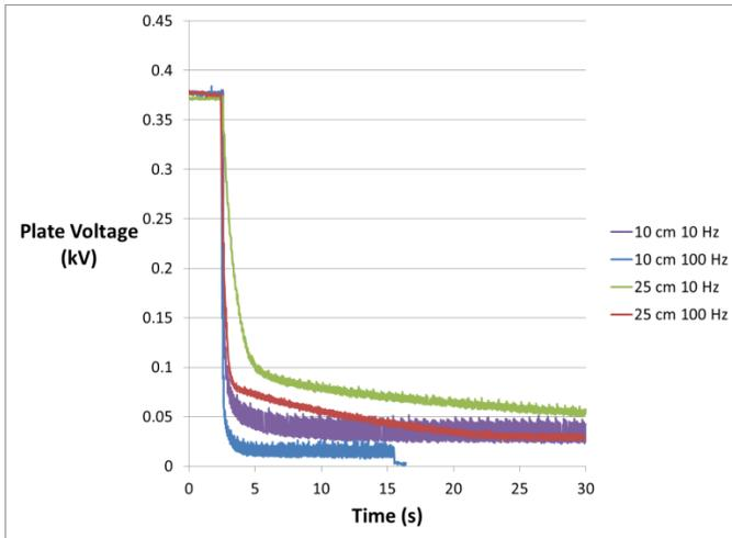
Fig. 12. Discharging a 180 pF capacitor in a simulated Martian atmosphere using two static eliminator waveform frequencies and two distances of the eliminator
