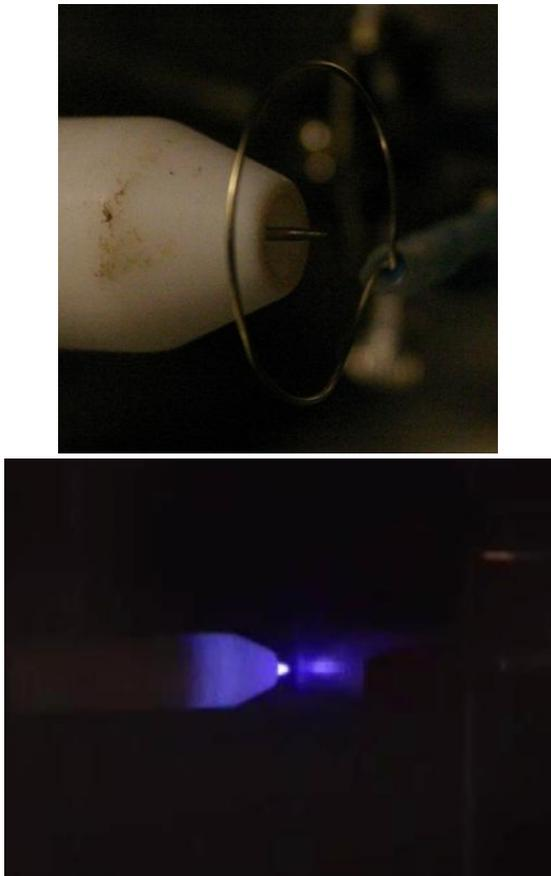
Fig. 10. Static eliminator geometry (Top), Static eliminator corona/glow discharge in a simulated Martian atmosphere (bottom)
