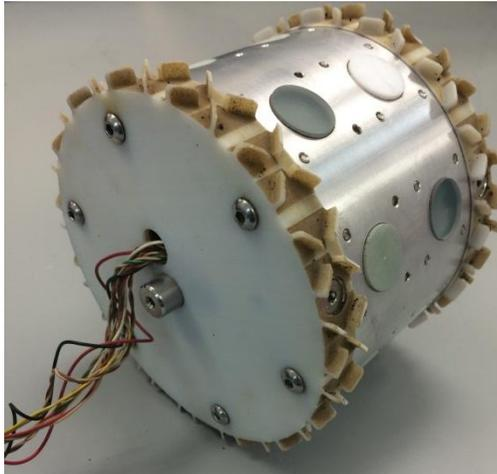
Fig. 3. Wheel Electrostatic Spectrometer second generation prototype
