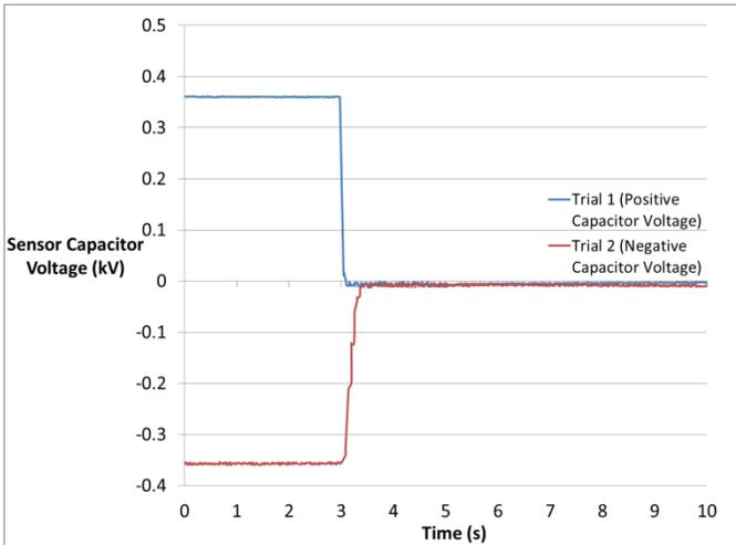
Fig. 14. Static elimination testing on WES sensor based capacitor in a simulated Martian atmosphere
