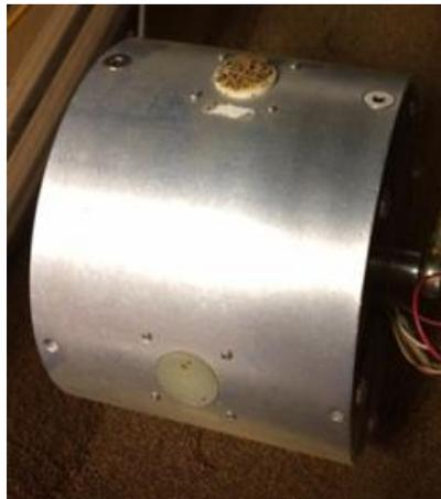
Fig. 9. Dust clinging electrostatically to Teflon (top center) and G10 (bottom center)
