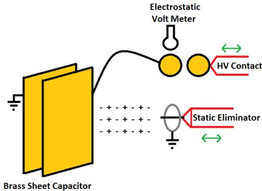
Fig. 11. Static eliminator test configuration
